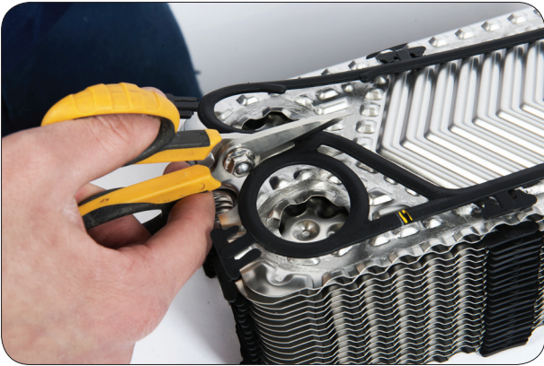
4.5 Cut two channel plate gaskets into half.
