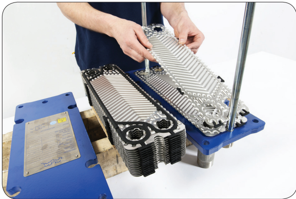
5.2 Assemble the plates according to the plate list of the configured heat exchanger.
