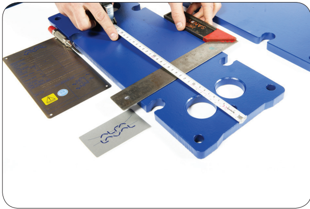
1.1 Place the sticker onto the frame plate according to the location sketch
