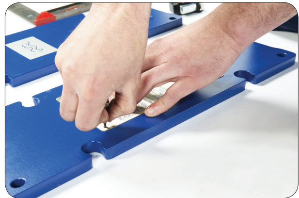
1.2 Mark the name plate position on the pressure plate according to the location sketch on page 6.
