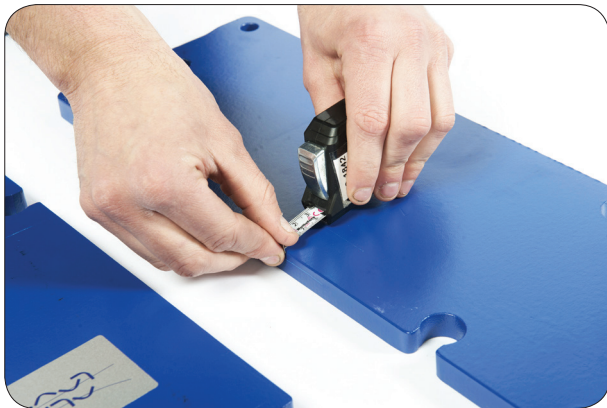
1.2 Mark the name plate position on the pressure plate according to the location sketch on page 6.
