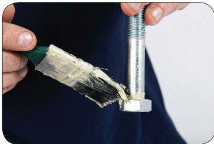
7.1 Grease the tightening bolts and nuts.
