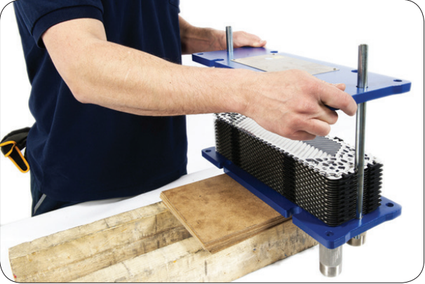
6.1 Put the pressure plate on the carrying bar while the unit is lying down.
