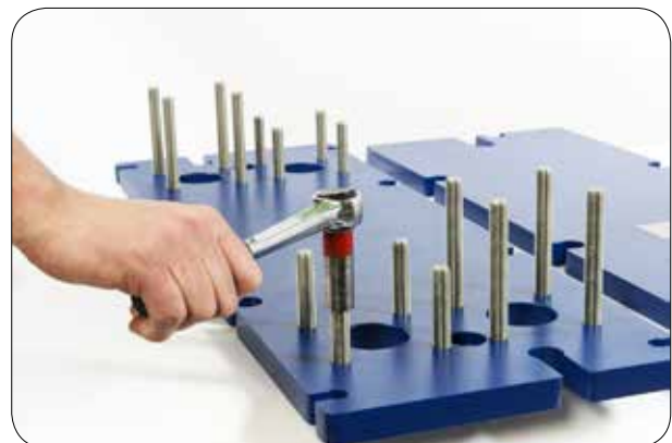
2.2 Screw the stud bolts until they reach the end of the threads in the frame plate.
