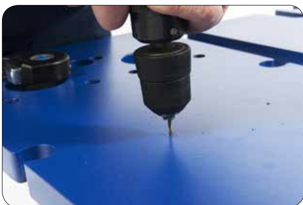
1.3 Drill four holes on the frame plate to fit the holes in name plate.
