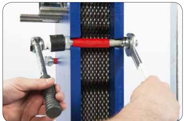
10.5 Tighten the bolts to reach the A-measure stated on the drawing of the heat exchanger.
