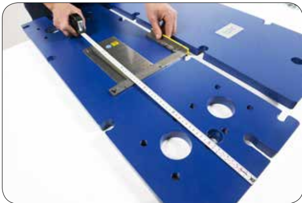
1.2 Mark the name plate position on the frame plate according to the location sketch on page 6.
