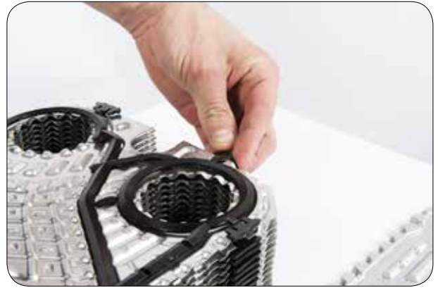
7.1 Assemble the gaskets onto the four-holed channel plate by using the fastening clips.
