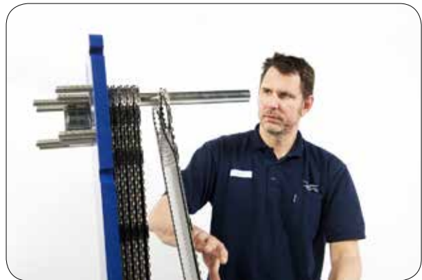
8.2 Hang the plates according to the plate list of the configured heat exchanger.
