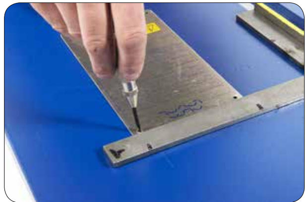
1.2 Mark the name plate position on the frame plate according to the location sketch on page 6.
