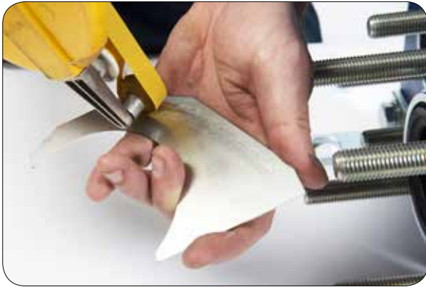
6.1 Apply glue onto the distance sheets and assemble the distance sheets around the linings on the frame plate's inside.
