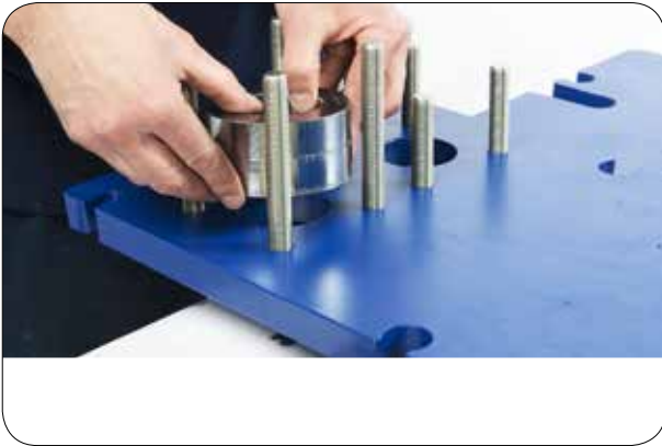
3.1 Position the distance rings according to the drawing of the heat exchanger.
