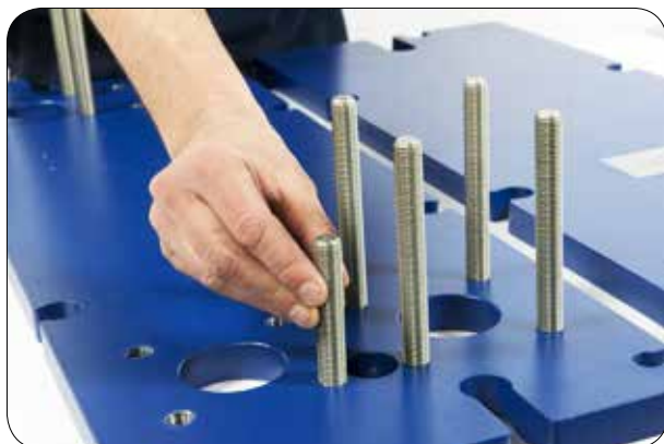
2.2 Screw the stud bolts until they reach the end of the threads in the frame plate.
