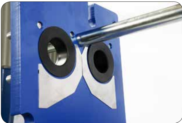
6.1 Apply glue onto the distance sheets and assemble the distance sheets around the linings on the frame plate's inside.
