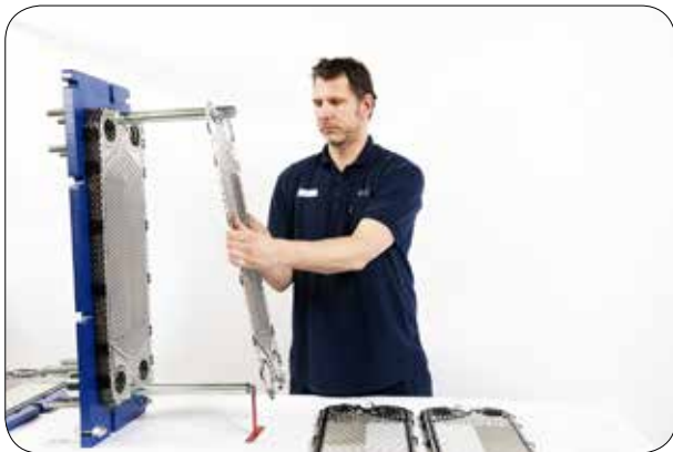
8.2 Hang the plates according to the plate list of the configured heat exchanger.
