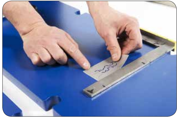
1.1 Place the sticker onto the pressure plate according to the location sketch.
