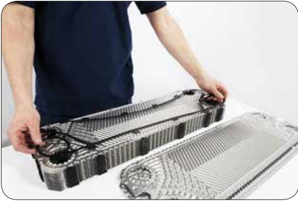
7.1 Assemble the gaskets onto the four-holed channel plate by using the fastening clips.
